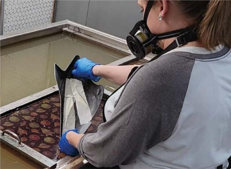
Hydrokon on water's surface prepared for dipping
